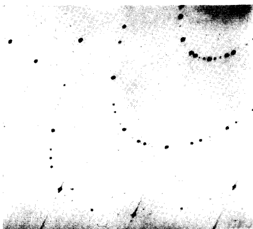
FIG. 2. Zero-layer Weissenberg pattern of YX_{2.11(5)} crystal (the 7F basic unit). Superstructure reflections are separated by one seventh of the distance between fluorite-type subcell reflections.
